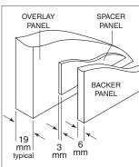
Panel assembly cross section. Panel assembly rear view.
